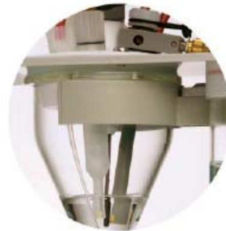
Rotating disk electrode (RDE) can be used in the same stand
