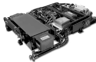
Figure 1.20 The 75-kW (approx.) fuel cell system for a prototype Mercedes Benz A-class car. (Photograph reproduced by kind permission of Ballard Power Systems.)
