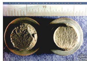
Hydrogen Embrittlement of Valve Capscrew Fasteners
